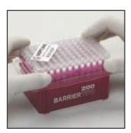
**4.** Secure plate by firmly pressing on all four corners of alignment plate
