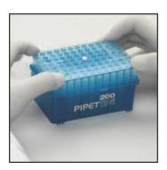
**3.** Secure plate by firmly pressing on all four corners of alignment plate
