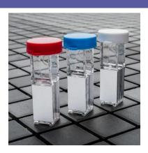
Genesee brand electroporation cuvettes' high-grade aluminum electrodes are produced through a unique manufacturing process which ensures a scratch-free surface for uniform pulse delivery to the entire sample. The 1mm cuvette has the narrowest gap and shallow bottom for small sample volumes (40-80 µl) and very high field strength, used for yeast and bacterial transformation. Comes with a distinguishing white cap. 1mm cuvette: minimum volume 20µl / maximum volume 90µl
